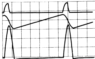
Kollektorstrom des Pulstran- sistors BU 111 (Rastermaß 2A/cm)
